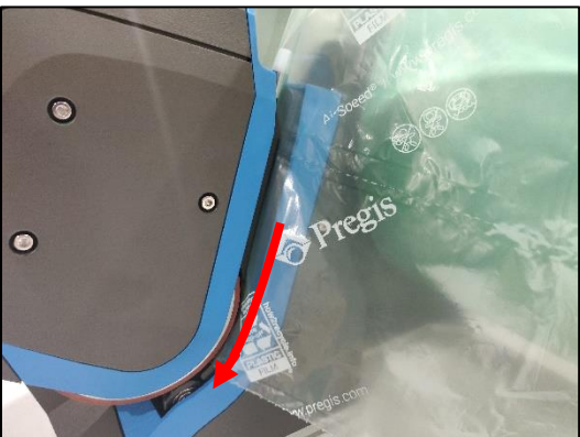
Figure 10. Pull the film forward to the Backing Wheel (larger, red wheel).
