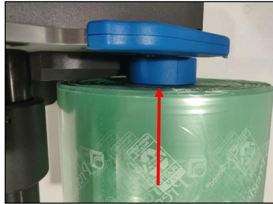
Figure 7. Firmly press the roll to the end of the Spindle, up against the flange.
